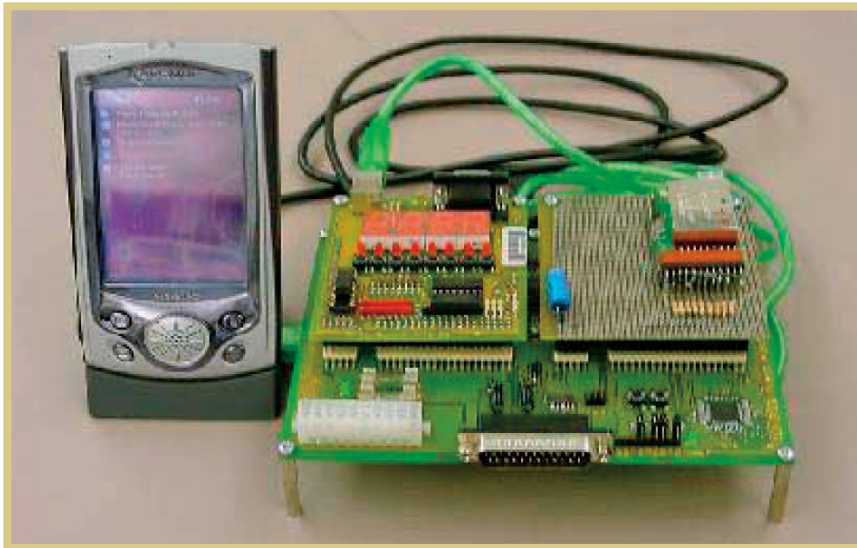
Figure 5. A PDA, equipped with our current RCSM prototype, for the Smart Classroom testbed. A software-only version of RCSM is currently under development.
