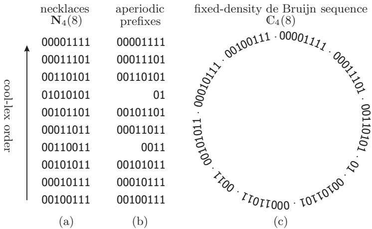
FIG. 6.1. Concatenating the aperiodic prefix in (b) of the necklaces of length 8 and density 4 in reverse cool-lex order in (a) creates the “cool-daddy” fixed-density de Bruijn sequence  $\mathbb{C}_4(8)$  in (c). The substrings of the cycle are the  $\binom{8}{4} = 70$  strings in  $\mathbf{B}_3^4(7)$ .
